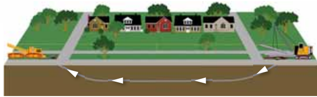
A guided boring machine creates an underground path, leaving the surface undisturbed.
